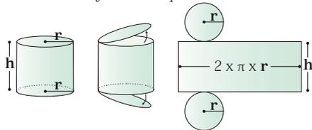
De la figura se infiere que:  $A_{\text{Cilindro}} = 2 \times \pi \times r^2 + 2 \times \pi \times r \times h$ .
